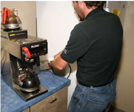
Plugging coffee maker into Kill-A-Watt meter
